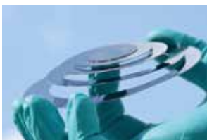
IV Ring of Si, shows the excellent bending strength and the possibility of resizing.
