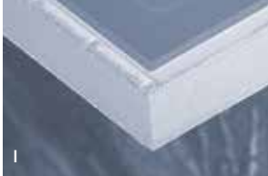
I SiC Wafer: free of chipping, backside-metal separated
